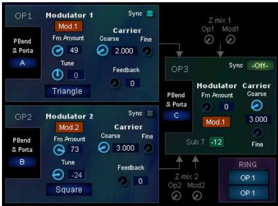
An operator is made of a “Carrier” sine Wave modulated by a “Modulator”.
