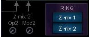
“Z-Mix” is an optional mix of the Operator and its Modulator. So it is the modulator running parallel to the FM operator (which is modulated by the same modulator). Using the Z mix by itself can give very fat sounds.
