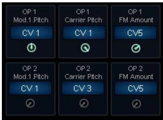
You can modulate the Pitch of the Modulator and the Carrier as well as the FM Amount.
