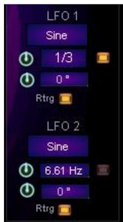
Make sure the Trigger buttons are “on” if you want to retrigger (on the picture attached, they are both off, ie, the LFOs are running freely and do not retrigger).
