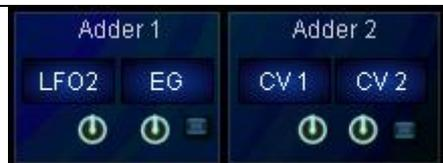
Allow to mix 2 modulation sources together. It includes the CV inputs and the internal modulators. The button at the right of one of the sources is an “inverse” button.
