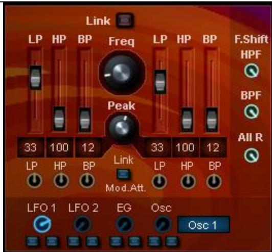
The “Peak” represent the maximum resonance possible. For example, in the above pic, LP is 33% of the peak pot, HP is 100% (same), and BP is 12% only (almost no resonance). The amount of “%” depends on the amount of “Peak”. If peak is at zero, then there cannot be any resonance.
