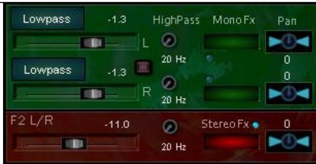
*Tip: The direct outputs of Spirit are taken after the Pan of each 3 channels of the filter mixer.*
