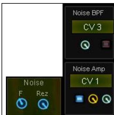
The Noise oscillator is a white noise with a 24dB resonant Bandpass.
