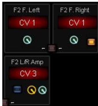
The formant filter modulator is the same for L/R channels. Stereo formant is achieved with the vowels and offsets rather than with CV modulators.
